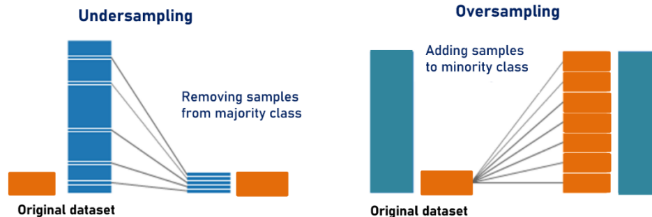
Fig. 3. Representative diagram of the two techniques: subsampling and oversampling
